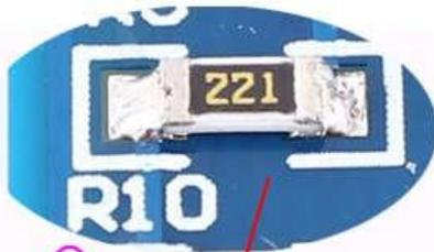
**Step 1:** Install 12pcs SMD 1206 Resistor at R1~R12.
